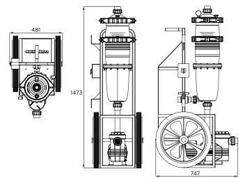
Note: Standard Ultravac comes with a 0.5Hp Supastream pump and Multicyclone Plus MC12 (40 ft<sup>2</sup> cartridge). Other combinations available upon request. Vacuum hose is not supplied.
