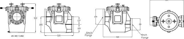
The Hydro5000 Commercial strainer is a corrosion resistant thermoplastic strainer designed for aquatic facilities, water parks and large commercial swimming pools.
