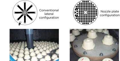
Internal Nozzle Plate Service Hatch
