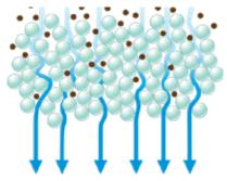
Glass Pearls operate on the basis of "depth filtration"; dirt is driven through the filter bed and trapped in minute spaces between the particles of filter media
