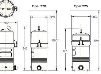
\* Minimum Clearance Height to Remove Cartridge (mm)
