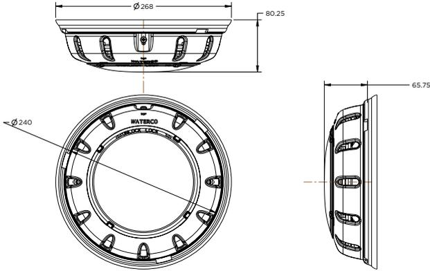
Waterco's Litstream LED Replacement Kit comes with a twist-lock adapter plate that can easily replace a majority of surface mount pool lights.
