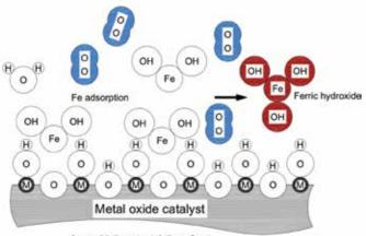
Iron oxidation at catalytic surface.
