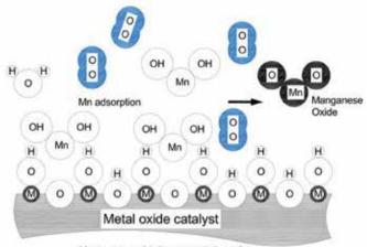
Manganese oxidation at catalytic surface.
