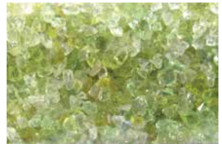
Ecopure glass has undergone specialised heat treatment process, which reduces degradation and therefore lengthens its life span.
