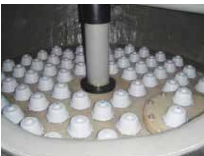
Micron SPDD filters incorporate a patented nozzle plate system which promotes uniform water flow when filtering and backwashing.
