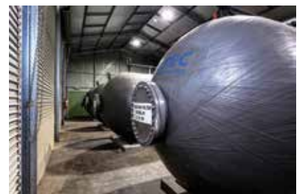
Fibreglass vessels have a mechanical and chemical resistance superior to steel, plus fibreglass does not rust or corrode and is able to withstand damage from many types of water treatment chemicals.
