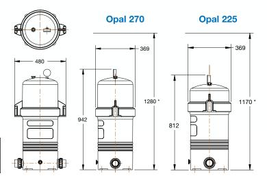
\* Minimum Clearance Height to Remove Cartridge (mm)
