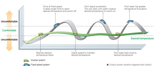
Electroheat ECO-V inverter pool heat pumps utilise a variable speed compressor to regulate the pool water temperature automatically and independently.
