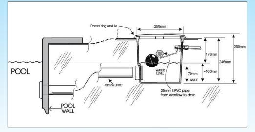
The Waterco Automatic Water Leveller is placed in the ground at a convenient location near the pool and plumbed to a separate pool inlet and also to the fresh water supply. The leveller remains inactive until the pool water level drops below or rises above the correct point at which time it will restore the right level by adding or draining water as the situation requires.
