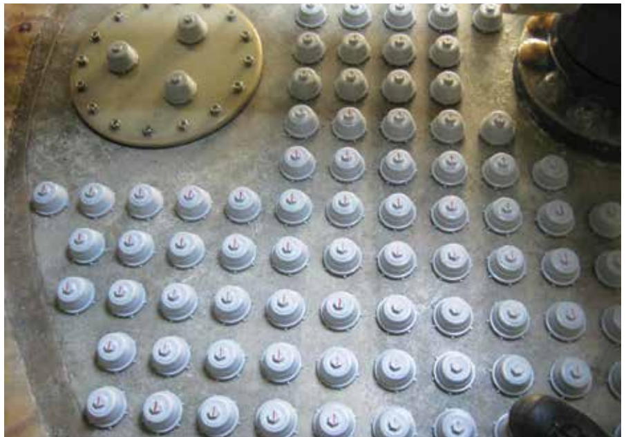
Waterco's patented method of fabricating a nozzle plate filter practically eliminates failure rates experienced in most other nozzle plate filters.
