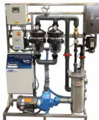
At the heart of the Reclaim system are twin commercial grade Waterco MultiCyclones that remove particulates from the water before sending it out to the car wash equipment.
