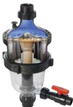
Waterco's award winning MultiCyclone is a brilliant pre-filtration device that works on the basis of centrifugal water filtration and is designed with no moving parts and no filter media to clean or replace.
