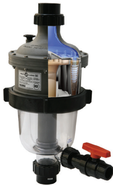
The MultiCyclone M16 is a pre-filtration device that works on the basis of centrifugal water filtration. There are no moving parts to wear and tear and no filter media to clean or replace.
