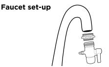
internal thread set-up
